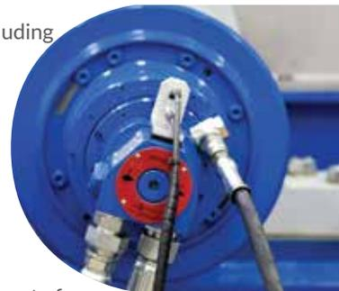
Refer to the *Centrisys Hydraulic Scroll Drive Brochure* to review advantages of a hydraulic back drive vs. the gear box design.
